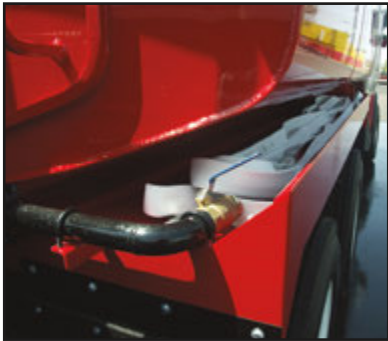
FENDER HOSE TRAYS Integrated fender hose trays for lay flat hose storage.
