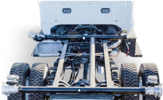
(A) The 3" rear spray bar tees into the supply line. (B) 3" manifold with grooved ends to be installed at a specified mid-ship location. The manifold pipe and rear bar pipe are mounted to the outside of the frame rail with bolt on brackets.
