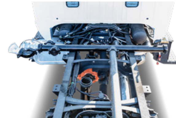
Top view of water pump mounted frame rail on driver side. Plumbed to manifold with rear supply pipe attached.
