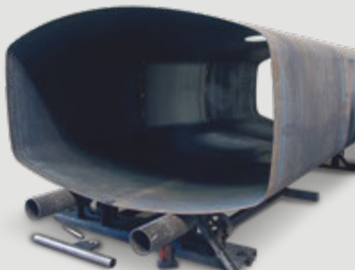
FULL PENTRATION WELDS INSIDE & OUT 100%
