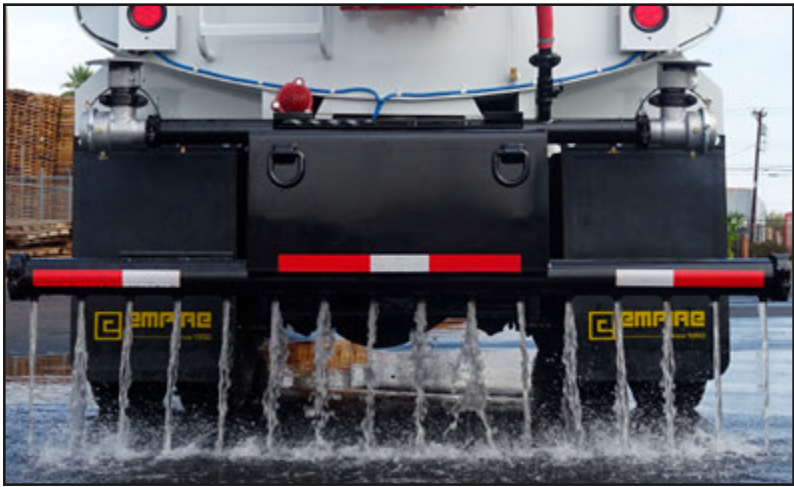
DRIP BAR KIT 8' Wide with 1/2" Female Threaded Ports on 6" Centers Optional Brass VeeJets Sold Separately Air Operated Butterfly Valve Plumb to Pump for Pressure or Tank for Gravity Spray
