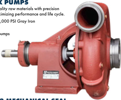
M3ZRMS 4X3 MECHANICAL SEAL UNITEDBUILT CAST IRON CENTRIFUGAL WATER PUMP 4X3 MAX RPM: 2,500 RATED: 750GPM @ 65PSI
