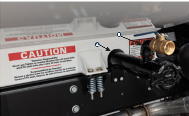
(A) Cut out arch in the tank runner for the manifold pipe mounted to the frame rail. (B) 1 1/2" brass jet valve mounted on passenger side of truck. Note the mounting bracket for the manifold pipe.
