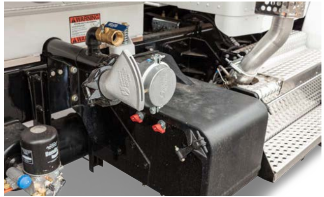
Optional 90° side spray valve on passenger side of truck (standard on stock tandem axle systems). Easily adjust 90° fitting and nozzle orientation for desired spray pattern and direction.
