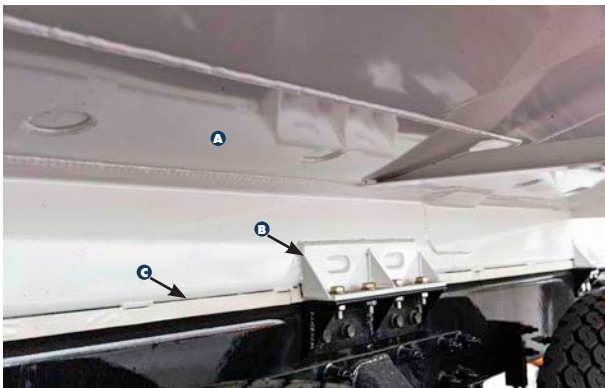
(A) Full length belly plate for tanks 3,000 gallons or more effectively doubling bottom tank thickness. (B) Extra duty bogie mounting brackets for tanks exceeding 4,000 gallons. (C) Vulcanized rubber wear pads welded to runners on tanks 3,000 gallons or more absorb vibration and increase the life of the tank. (See mounting instructions page 57.)
