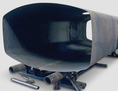
FULL PENETRATION WELDS INSIDE & OUT 100%
