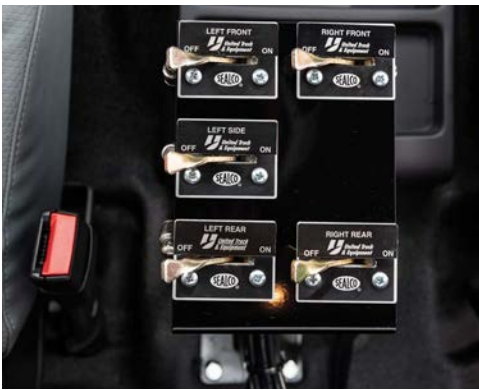
Spray valves are independently controlled with in the in cab mounted control tower. Each switch is plumbed with 1/4" airline to a spray valve for independent control.
