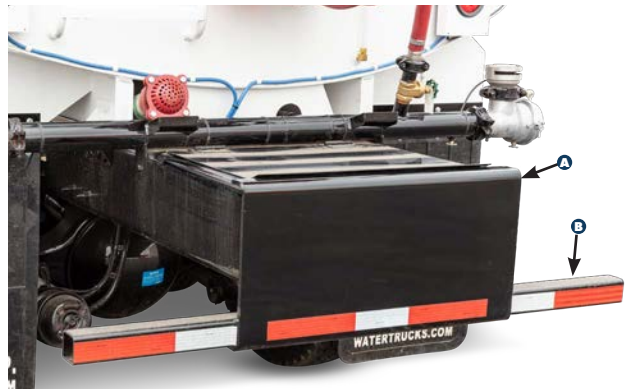
(A) Push plate is constructed of 1/2" steel with internal storage and lid. (B) Drive under protection is constructed from 3x3" square tubing welded to the push plate.
