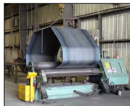
SHELLS ROLLED WITH MINIMUM THICKNESS \frac{3}{16} " A36 SHEET STEEL
